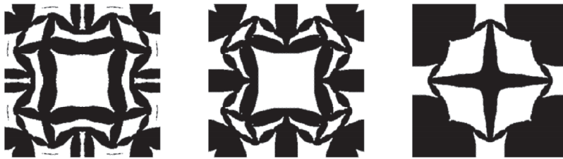
FIG. 7. Poisson ratio minimization: RVE for \alpha = 0 (left), \alpha = 0.01 (middle), and \alpha = 0.02 (right). The corresponding Poisson ratios are -0.345 , -0.319 , and -0.260 , respectively.
