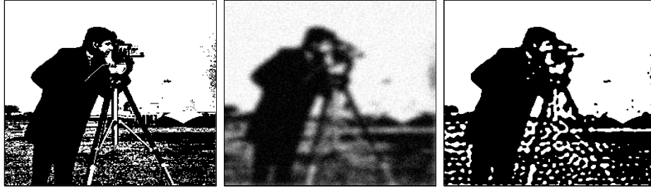
FIGURE 15. Deblurring and denoising, from left to right: original image (left, 257 \times 257 pixels), damaged image with blur and noise effects (middle), reconstructed image for \alpha = 2.10^{-4}\sqrt{n} (right).
